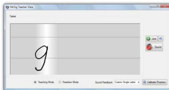
Figure 3. The teacher view of McSig, showing lines that are calibrated to the position of the student's tactile lines.
