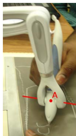
Figure 2. Point A is moved about the trajectory and the student can rotate the pen about the axis indicated.
